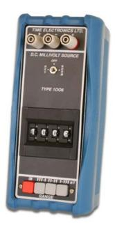
The **1006** is an accurate low cost millivolt source suitable for voltage injection applications. Three output ranges are provided to give adjustable output values from  $1\mu V$  to 1V with a basic 0.02% accuracy. For signal injection, the operator needs to switch on, check the battery condition, select the range, and set the required voltage using the thumbwheel switches. The 1006 uses a precision reference diode and low temperature co-efficient resistors to give a highly stable output.
