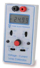
The **1048** is a current, voltage, and process loop calibrator that covers the needs of an R&D lab and process control engineer. Source and measure in three current and voltage ranges plus a transmitter simulator/sink function. It has 4.5 digit (0.005% of span) resolution.
