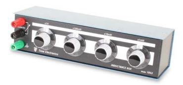
The **1053** is a compact, robust and accurate decade inductance box suitable for filter design, experimental, general purpose substitution, and DC to DC converter design.
