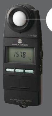
Receptor diffuser window: Ø **25** mm
