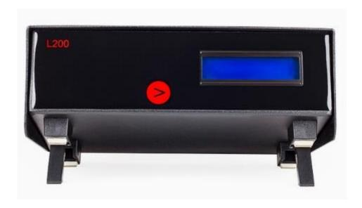
The Labfacility L200 Pt100 and thermocouple thermometer can be used in conjunction with a PC to provide accurate, versatile 8 channel thermocouple and Pt100 temperature measurement, scanning and logging of measured values. It can also be used as a "stand alone" indicator/logger and incorporates a digital display of measured temperature.
